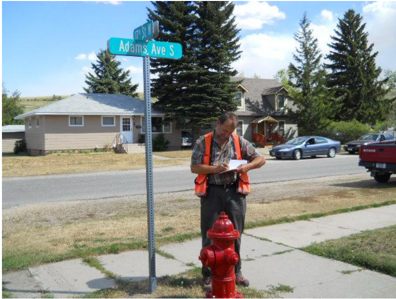
8/22/2011 2:56:08 PM View southeast of temporary benchmark on fire hydrant Street corner, Red Lodge, MT 2011-0057.JPG
